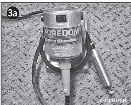
3a. At Ocutech, we use an industrial Foredam Flexible Shaft Grinder...
