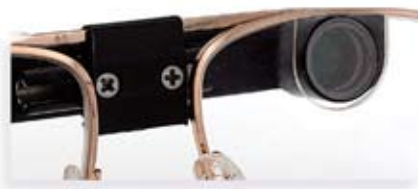
Carrier lens is slotted to allow eyepiece to pass through.
