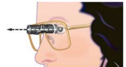
Simply drop the head and look into the eyepiece to sight through the telescope
