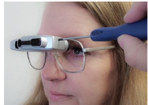
Eyepiece is easily adjustable for refractive errors
