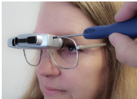
Eyepiece is easily adjustable for refractive errors
