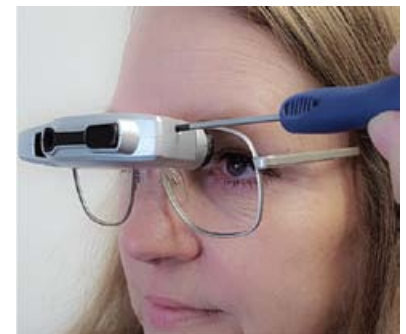
Eyepiece is easily adjustable for refractive errors
