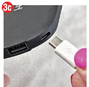
USB-C cable connected to Falcon (do not remove)
