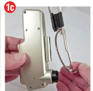
**3. Connect the USB cable to the battery**
