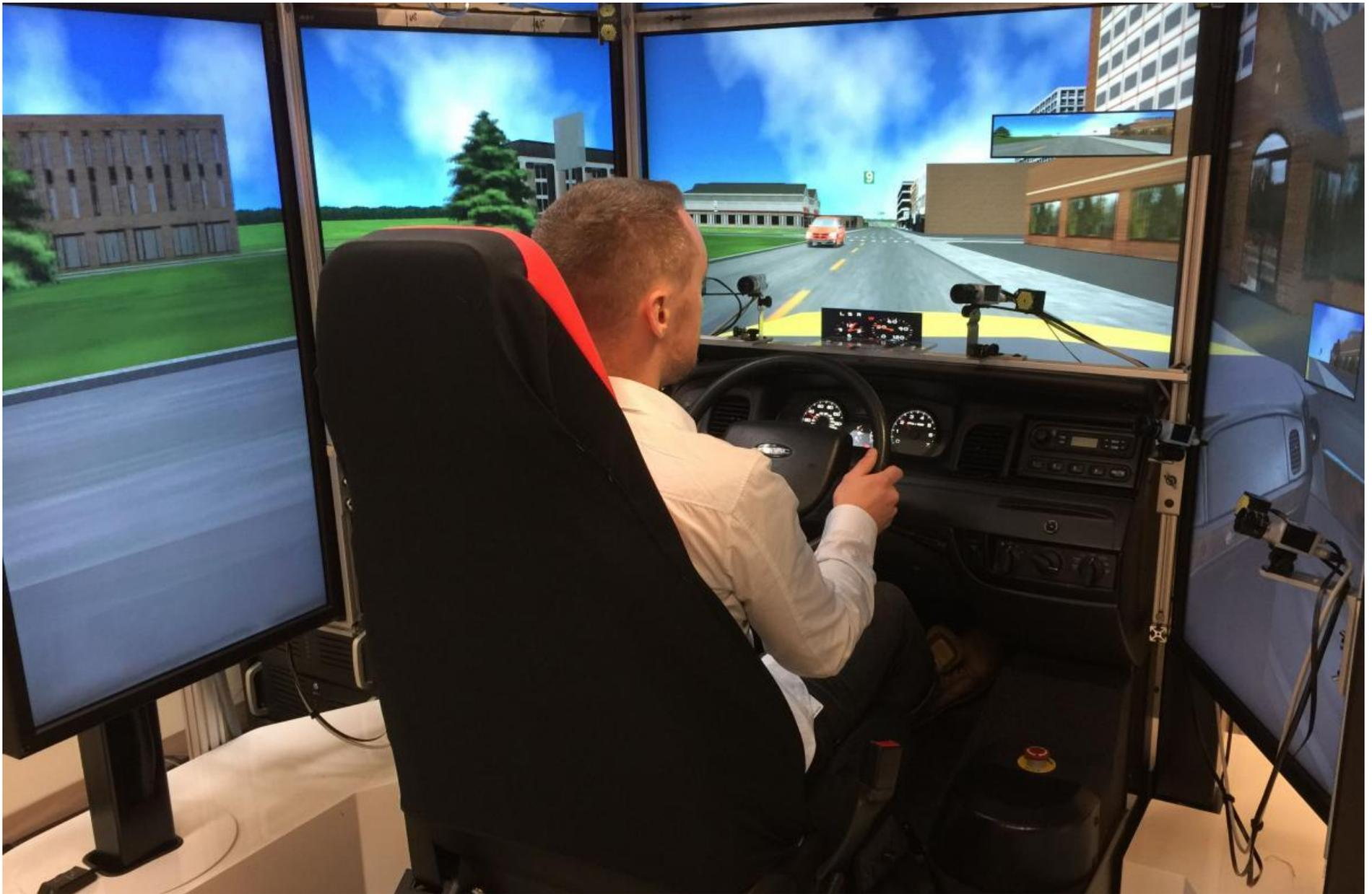
*Driving simulators enable researchers to study potentially dangerous driving situations*
